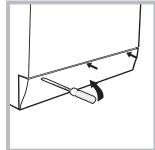
2. make sure the water level inside the machine is lower than the door opening; if it is not, remove excess water using the drain hose, collecting it in a bucket as indicated in the figure.
